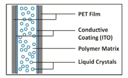
The liquid crystal privacy film is made up of electrically conductive coatings, a polymer matrix and liquid crystals. This film has electrical wiring to be connected to a transformer to supply power for the "on" (clear state) mode.
